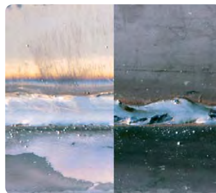
Descaled surfaces prior to welding lead to clean welding seams
