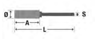
Zinc-plated twisted shaft with brass stabilising sleeve.
